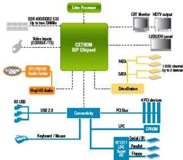
**Figure 2** An entire embedded computing and communications system with maximum system power of under 10W can be built using highly integrated CPUs and core logic silicon based on the latest 90 nm process technology, such as VIA Technologies' 500 MHz VIA Eden ULV processor and the VIA CX700M single-chip system media processor.
