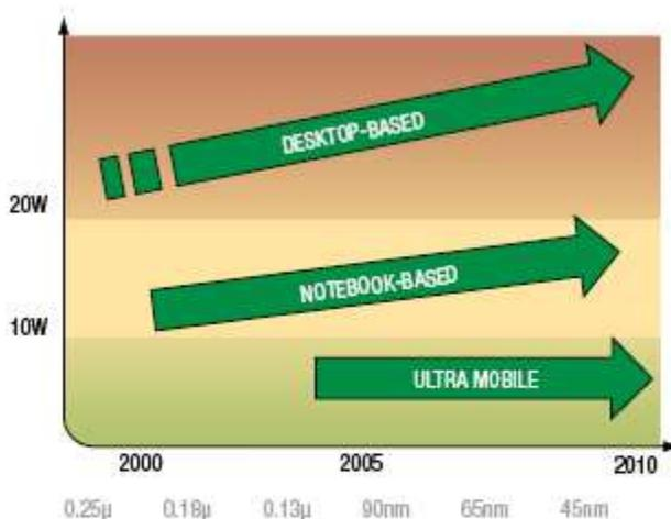
**Figure 1** Smaller chip geometries are making possible a new class of lower-power, ultra-mobile compute platforms that prioritize longer battery life and smaller footprint over processor performance.
